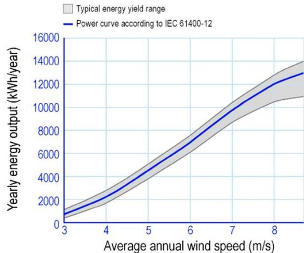
Data measured according to IEC 61400-12 standard
